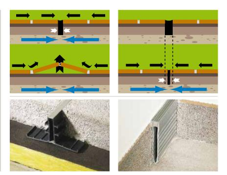
Any movement joints in the building structure must be carried through the tiling layer.
