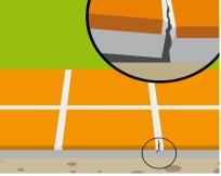
Tiling onto under floor heated systems; the tiles usually have a lower coefficient of thermal expan-sion. For a given temperature rise tiles will expand less than the substrate and stresses will be formed at the interface between the tile and the adhesive. At weak bonded parts, the tiles may delaminate or blow away from their base.
