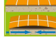
The grouting materials filled into joints should be flexible sufficient to absorb the movements occur-ring in horizontal with the surface. Too stiff grouting materials will fracture or depart from the tiles' edges
